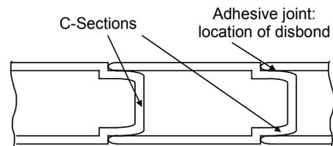
Figure 3 Typical helicopter rotor blade; detail of the blade cross-section indicating the adhesive joining of C-sections
