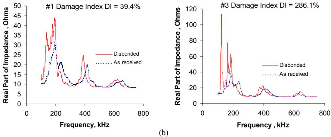
Figure 13 Comparison of the E/M impedance response curves measured for the “as received” and “disbonded” structure shows clear identification of the disbond: (a) spectrum of the disbond gauge at location #1; (b) spectrum of the disbond gauge at location #3.
