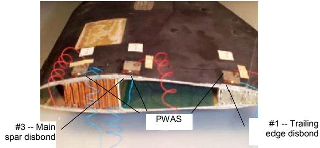
Figure 12 Piezoelectric active wafer sensors were used on a rear-rotor blade section to detect delamination between the adhesively bonded structural elements
