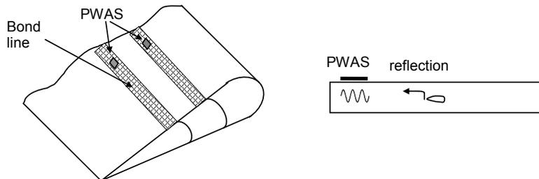
Figure 5 Pulse-echo method for damage detection
