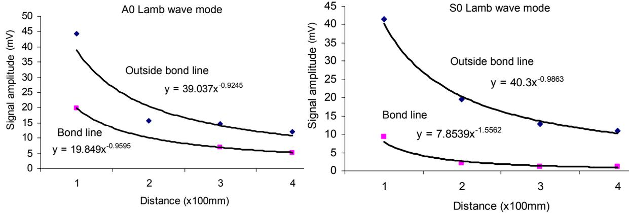
Figure 9 Attenuation of the (a)  $A_0$  mode Lamb waves traveling along the bond line; (b)  $S_0$  mode Lamb waves traveling along the bond line
