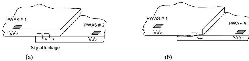
Figure 4 Pitch-catch method for joint inspection: (a) pristine joint carries the signal well from PWAS # 1 to PWAS # 2 through “leakage”; (b) Disbonded joint cannot carry well the signal resulting in degradation of signal received at PWAS # 2
