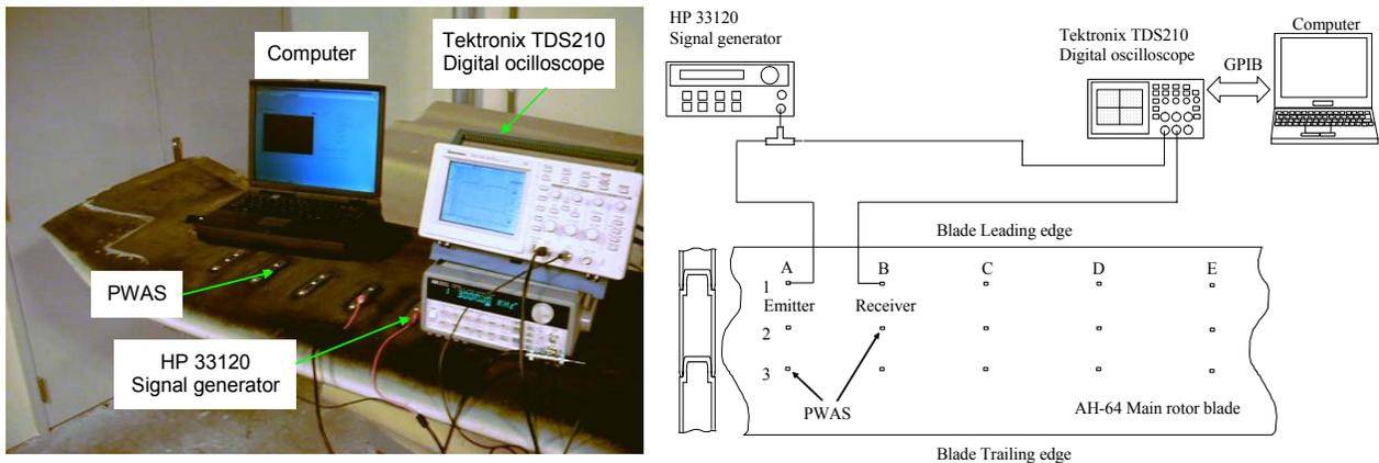
Figure 6 Schematic of the instrumentation setup
