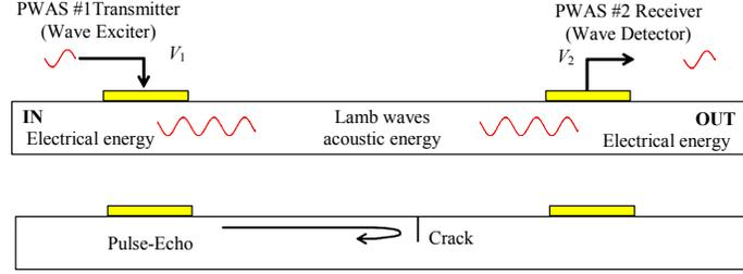
Figure 1 Ultrasonics damage detection techniques with the pulse-echo method
