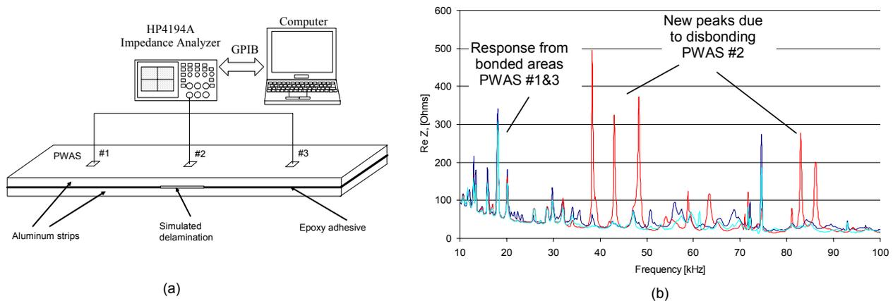
Figure 11 The aluminum bonded specimen: (a) experimental setup; (b) the E/M frequency response measured in three locations
