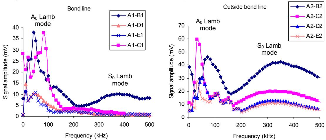
Figure 8 Lamb waves traveling (a) along the bond line; (b) outside the bond line
