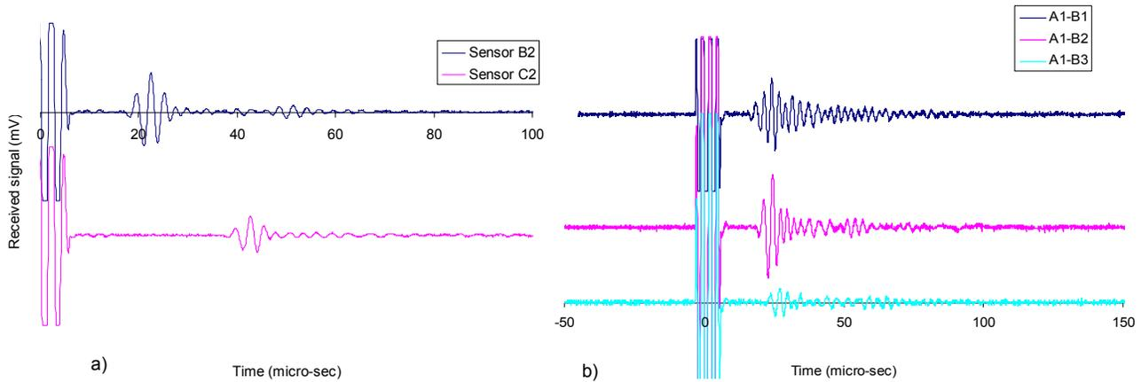
Figure 7 (a) Surface-guided Lamb waves received at (a) sensors B2 & C2 (100 mm apart) when excited from sensor A2 along the bond line (b) received at sensors B1, B2 & B3 when excited from sensor A1 across the bond line
