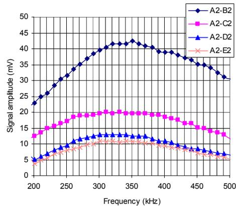
Figure 10 Optimal frequency band for transmitting and receiving surface Lamb waves
