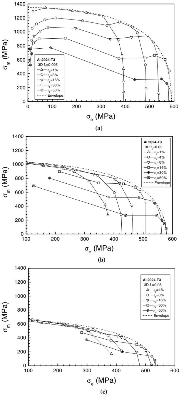
Fig. 6 Three-dimensional simulation results at void link-up for (a)  $f_0 = 0.005$ ; (b)  $f_0 = 0.020$  (c)  $f_0 = 0.080$ .
