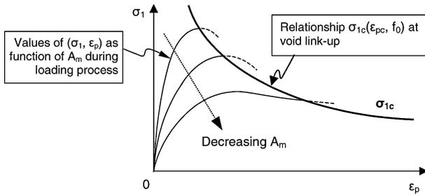
**Fig. 13** Relationship between plastic limit-load stress  $\sigma_{1c}$  and critical effective plastic strain  $\epsilon_{pc}$  for a specific  $f_0$ .
