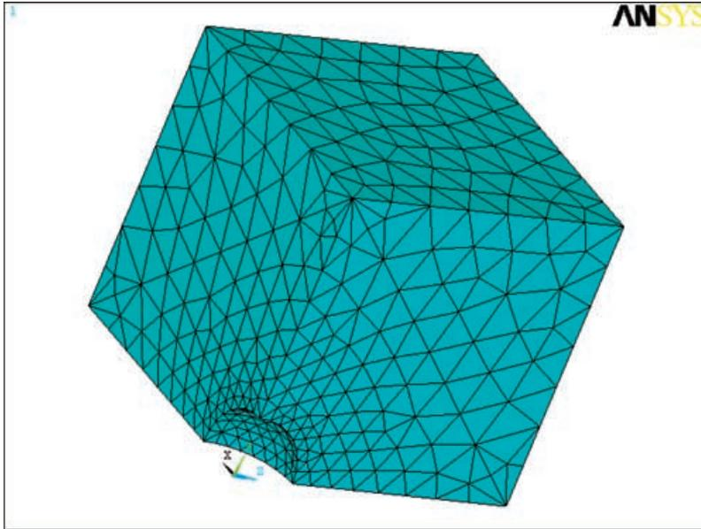
Fig. 4 One-eighth model for 3D unit cell.
