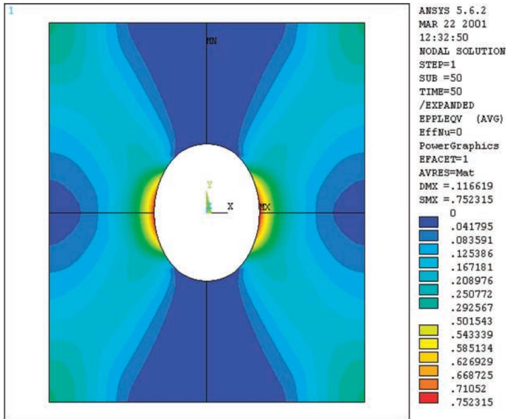
Fig. 12 Typical shape of plastic zones at link-up for low constraint.
