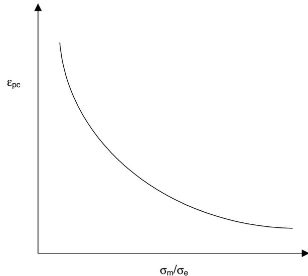
Fig. 1 Typical relationship between critical plastic strain and constraint.
