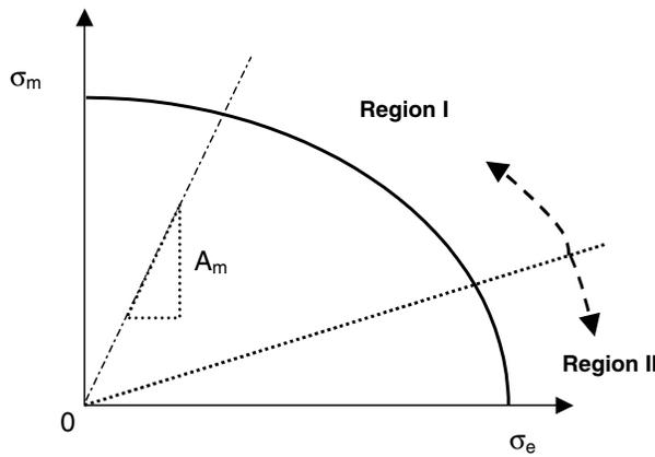
**Fig. 14** Schematic of Regions I and II for  $(\sigma_m, \sigma_e)$  envelope with void volume fraction  $f_0$ .
