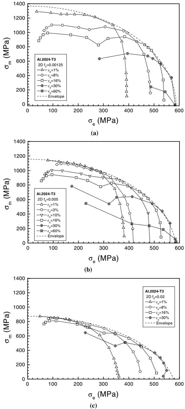
Fig. 5 Two-dimensional simulation results at void link-up for (a)  $f_0 = 0.00125$ ; (b)  $f_0 = 0.005$  (c)  $f_0 = 0.020$ .
