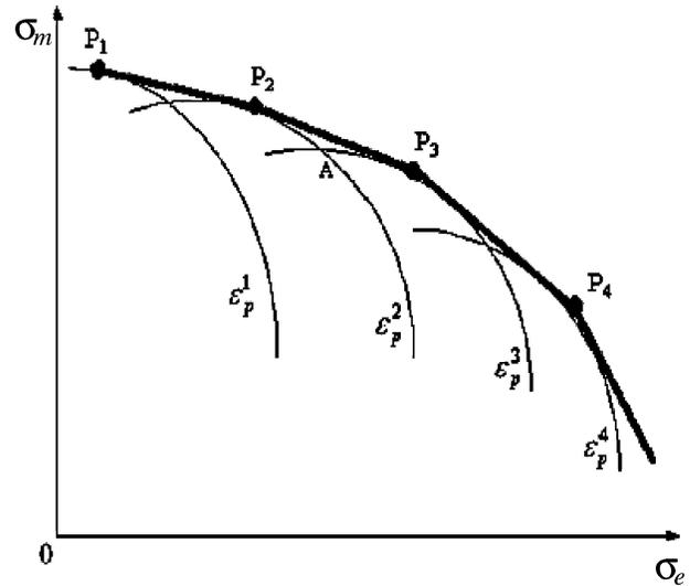
Fig. A1 Schematic for determining  $(\sigma_m, \sigma_e)$  at failure initiation.
