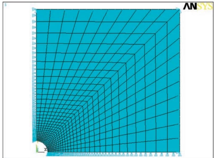
Fig. 3 One-quarter model for 2D plane strain unit cell.
