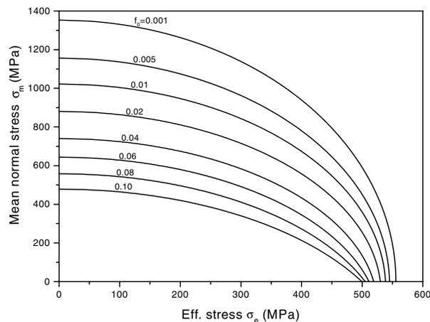
Fig. 10 Envelope functions  $\sigma_m$  and  $\sigma_e$  for each  $f_0$ .
