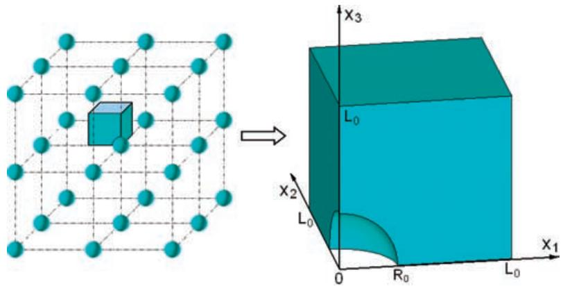
Fig. 2 Three-dimensional periodic array of voids and unit cell material model.
