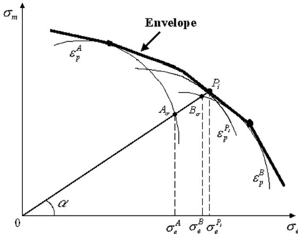
Fig. A2 Illustration of basis for maximum effective stress criterion.
