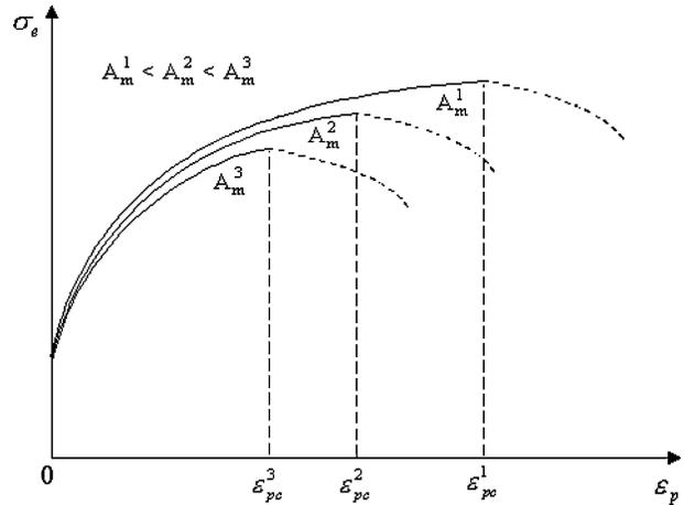
**Fig. 9**  $\sigma_e$  versus  $\epsilon_p$  as a function of  $A_m$  for a typical void volume fraction,  $f_0$ .
