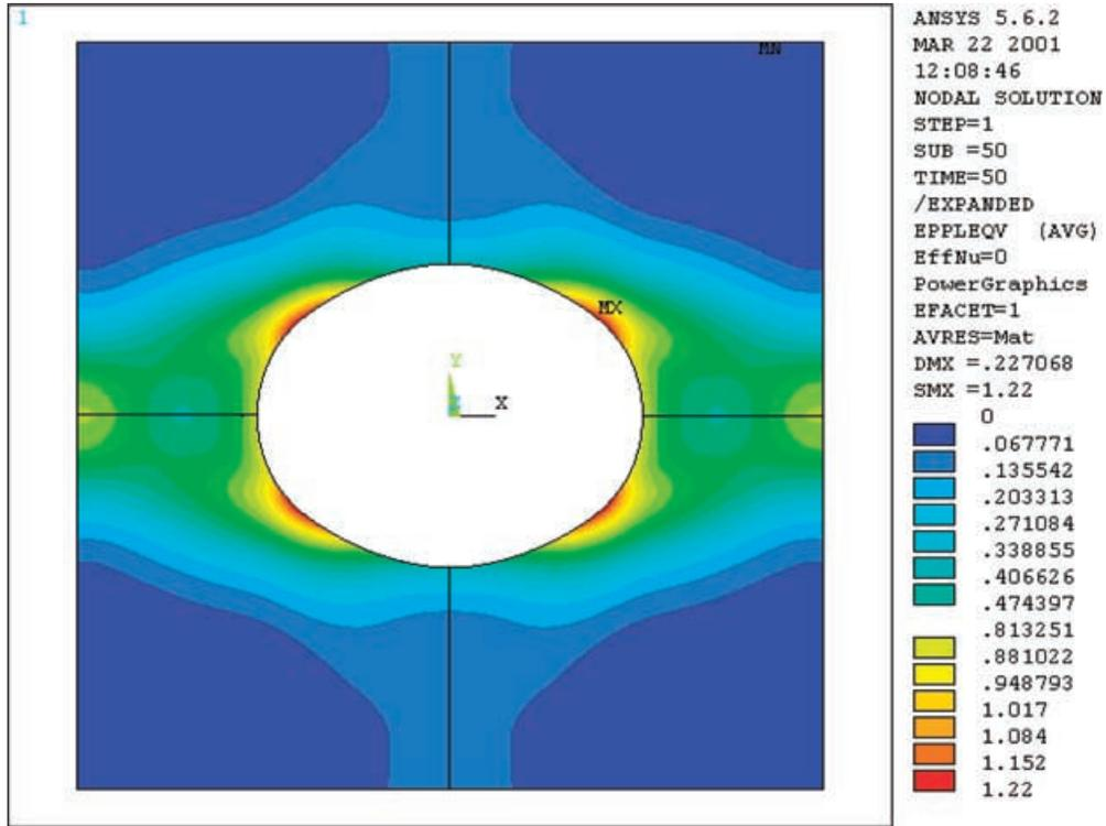
Fig. 11 Typical shape of plastic zone at link-up for high to moderate constraint.
