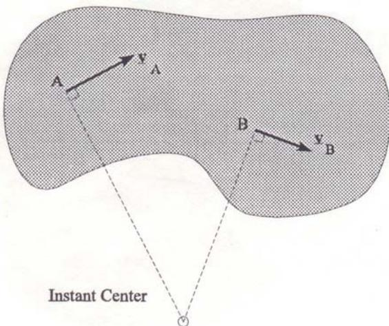
To find the instant center for a single body when the velocities of 2 points are known we take advantage of the fact that the linear velocities of all points in a rotating body are perpendicular to their radii of rotation.
