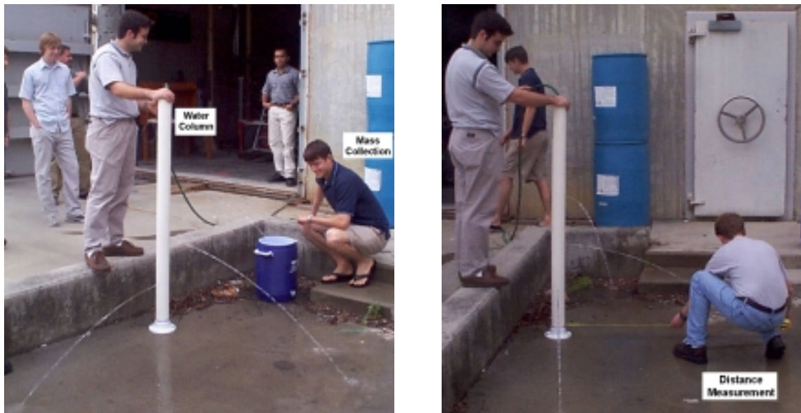
Figure 2. In the Head Pressure laboratory, freshmen determine flow velocities from mass and time measurements, distance measurements, and the Bernoulli equation.
