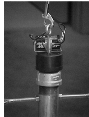
Figure 7: Electromagnet on yoke
