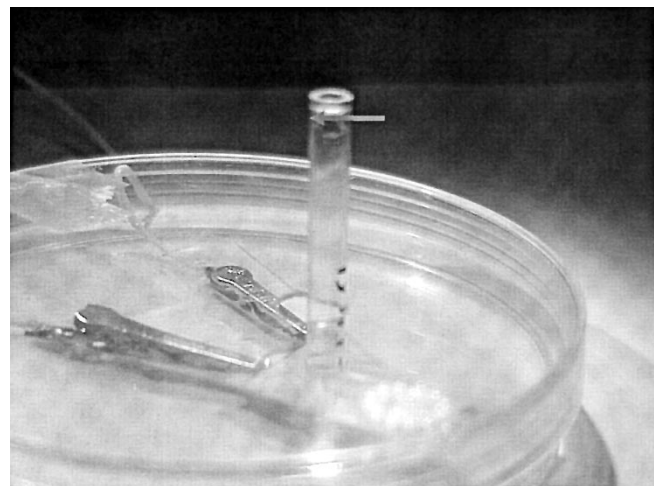
Fig. 5. Static pressure test of device (Liquid column level is near the top of tube).
