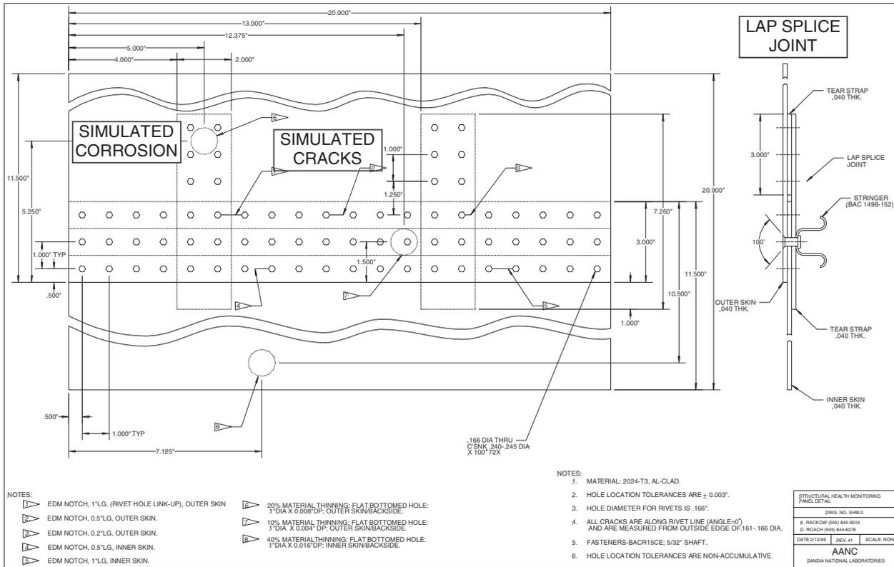
**Figure 2** Blue print of the experimental panels developed at Sandia National Laboratories as specimens for testing active-sensor structural health monitoring, damage detection, and failure prevention methodologies. The specimen has a built-up construction typical of conventional aircraft structures. It contains simulated cracks (EDM hairline slits) and simulated corrosion damage (chem.-milled areas).
