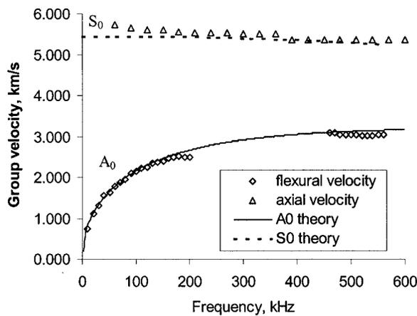
**Figure 9** Group velocity dispersion curves for Lamb-wave  $A_0$  and  $S_0$  modes.
