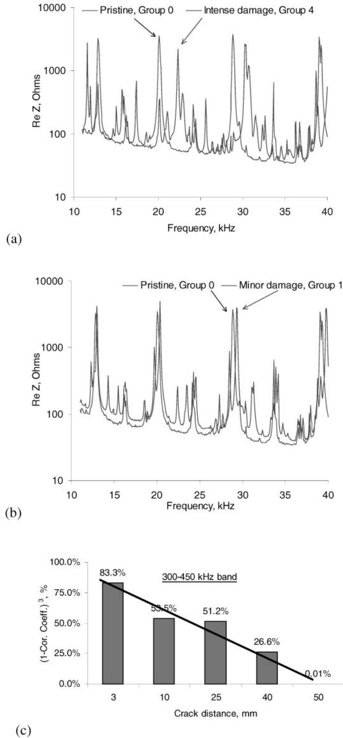
**Figure 5** E/M impedance results: (a) superposed groups 0 and 4 spectra (10–40 kHz band); (b) superposed groups 0 and 1 spectra (10–40 kHz band); (c) damage metric variation with the distance between the crack and the sensor (300–450 kHz band).
