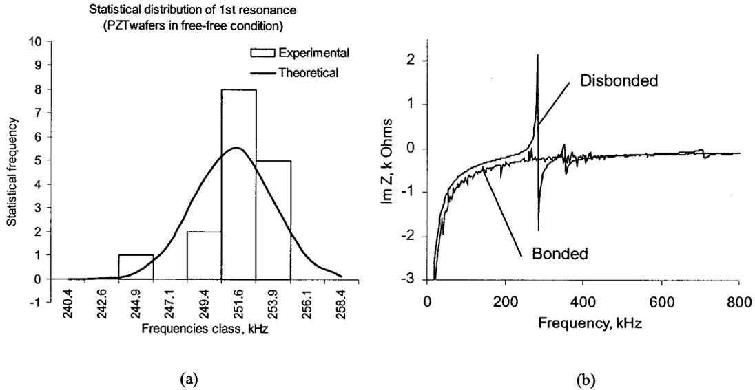
**Figure 3** PWAS calibration and self-diagnostic: (a) statistics of a PWAS batch showed consistency of first-resonance from  $\text{Re } Z$  measurements; (b) PWAS self diagnostic with  $\text{Im } Z$ : when sensor is disbonded, a new free-vibration resonance appears at 267 kHz.
