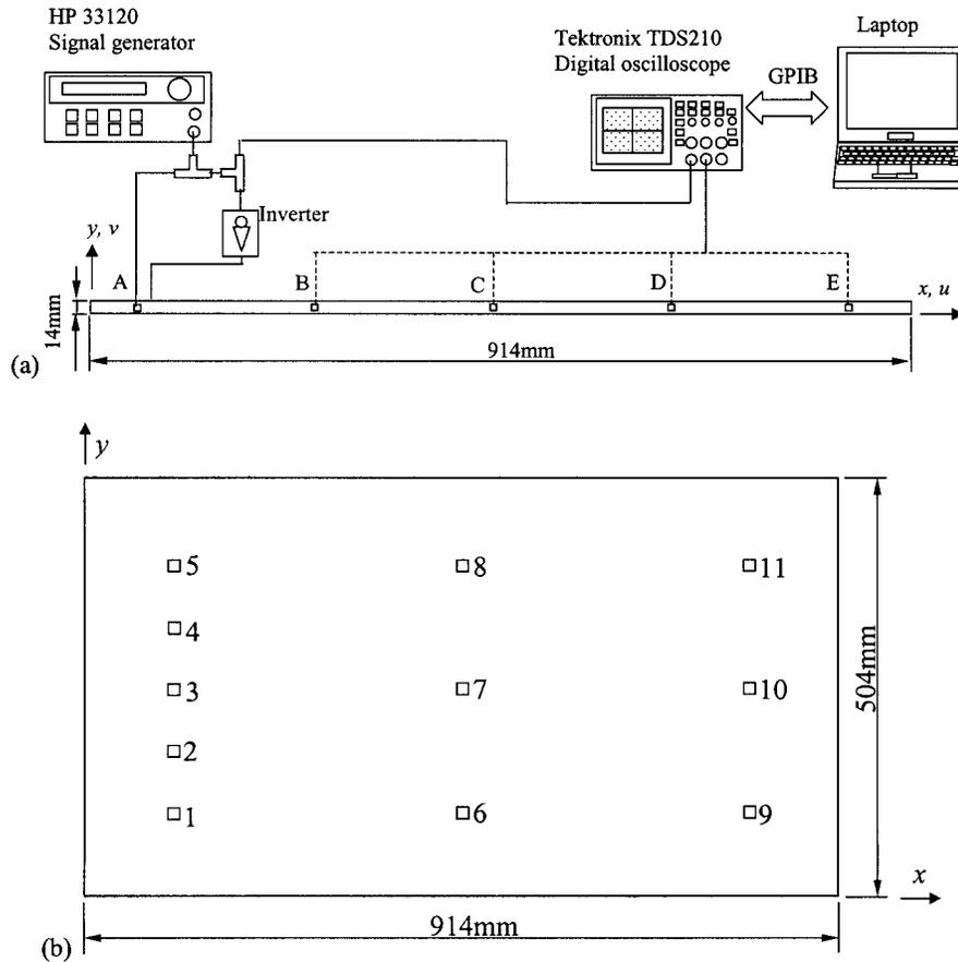
**Figure 7** Simple geometry specimens: (a) narrow strip beam specimen of 1.6 mm thick 2024 aluminum alloy, 14 mm wide and 914 mm long. Shown are the five pairs of piezoelectric wafer active sensors (A through E); (b) rectangular plate specimen of 1.6 mm thick, 2024 Aluminum alloy, 504 mm wide and 914 mm long.
