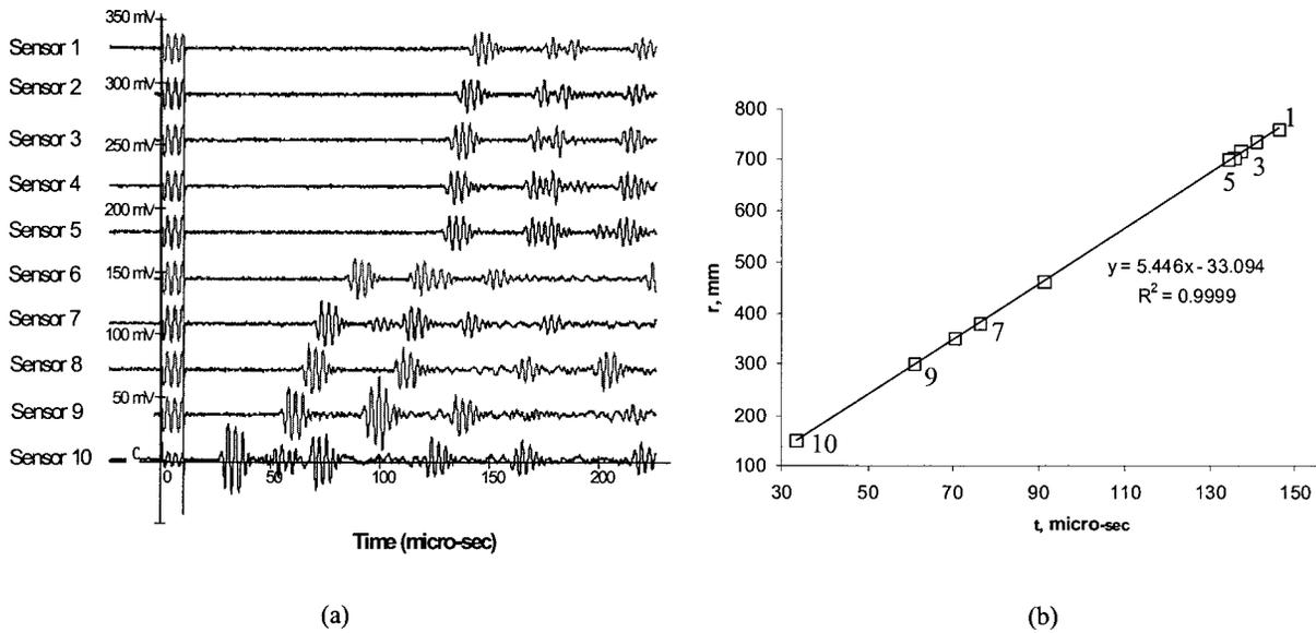
**Figure 10** Signals observed during the rectangular plate experiments: (a) raw reception signals received at active sensors 1 through 10 when sensor 11 was excited with a 300 kHz smoothed tone burst; (b) time–distance correlation yields the wave group velocity with remarkable accuracy.
