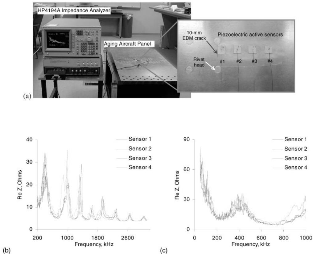
**Figure 6** Detection of crack damage in aging aircraft panels using PWAS and the E/M impedance method: (a) Four PWAS placed at increasing distance from a 10-mm simulated crack (hairline EDM slit); (b) Re Z spectrum in the wide frequency band, 200–2600 kHz; (c) Re Z spectrum in the narrow frequency band, 50–1000 kHz.
