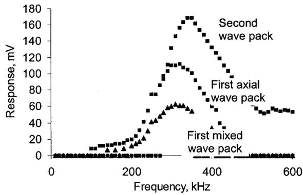
**Figure 8** Frequency tuning studies identified a maximum wave response around 300 kHz.
