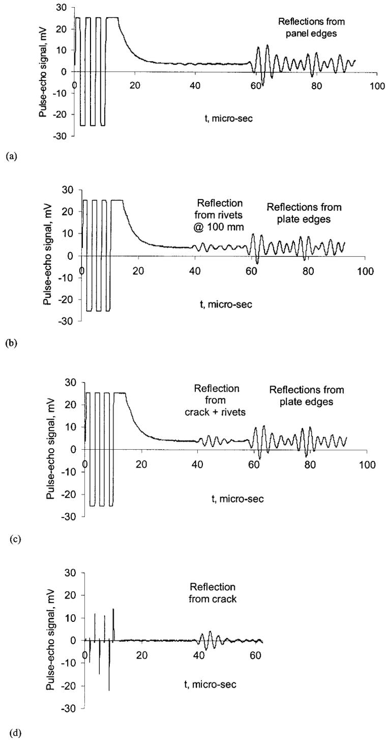
**Figure 13** Analysis of the pulse-echo signals for crack detection: (a) signal showing only reflections from the panel edges; (b) signal recorded in the pristine panel featuring the reflection from the rivets and from the panel edges; (c) signal recorded on the cracked panel featuring, in addition, the reflections due to the presence of the crack; (d) signal difference revealing the strong reflection from the crack.
