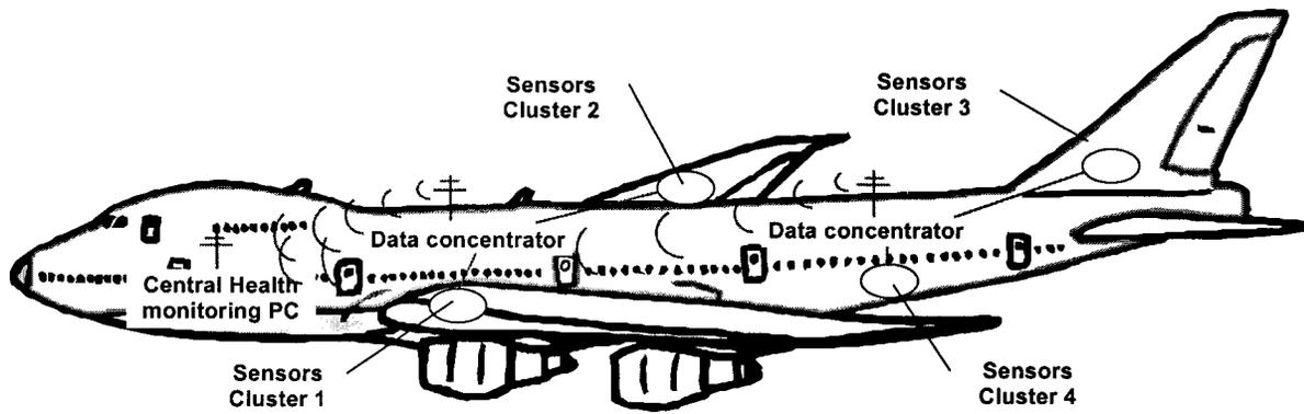
**Figure 14** General concept of a sensor-array structural integrity monitoring system suggested installation on an aging aircraft.
