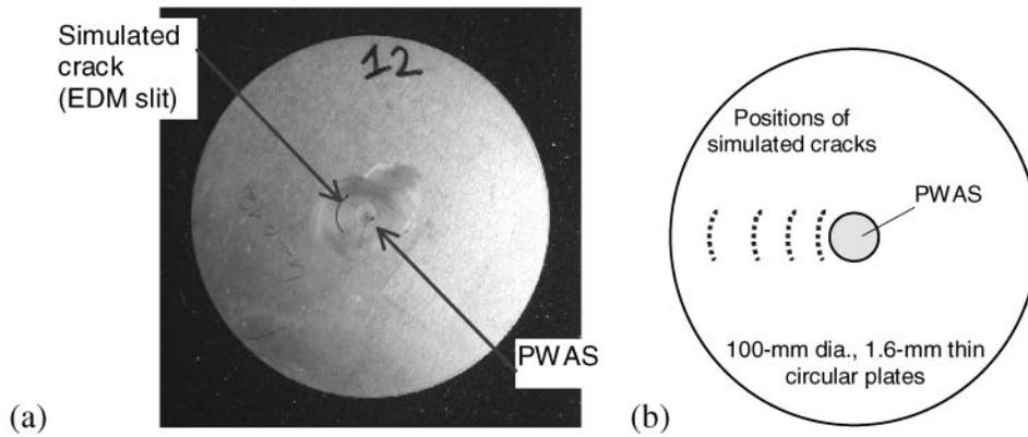
**Figure 4** Systematic study of E/M impedance technique on circular plates: (a) Photograph of actual specimen showing a 7-mm piezoelectric-wafer active sensor (PWAS) and a simulated crack (EDM slit); (b) progression of specimen geometries with simulated cracks (slits) at decreasing radial distances.
