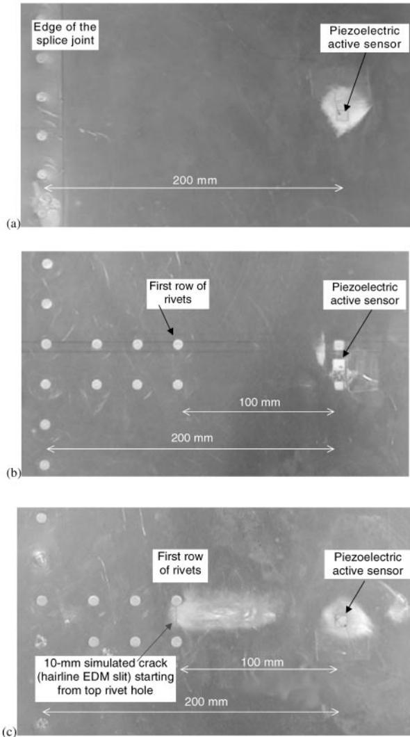
**Figure 12** Crack detection experiment on aging aircraft panel: (a) pristine panel featuring an active sensor placed in a rivet-free region; (b) pristine panel featuring an active sensor placed at 100 mm from a row of rivets; (c) damaged panel featuring a 10 mm simulated crack (hairline EDM slit) starting from the top rivet.
