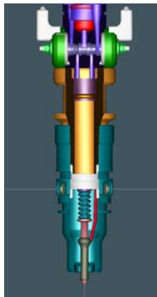
Fuel injector designed for the envisioned hydrogen-powered engine.
